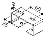
Width of the hole to be made in the false ceiling: **13 cm.**
