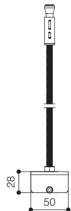
The **SLOPING CEILING** brackets for the Screen Winch System have been developed in order to mount the screen winch housing onto a wall or a sloping ceiling. The brackets can be tilted at any desired angle to adapt them to the sloping ceiling.
