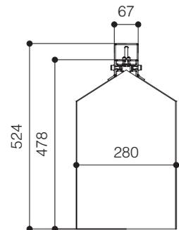
**NOTE:** The left and the right anchoring points have to be fixed at the same distance from each end side of the cabinet. The fixing distance has to be maximum 50 cm from left and right end sides of the cabinet.
