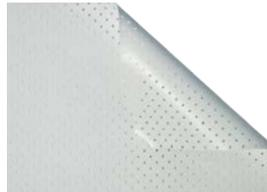
**MICROHOLES** cloth is made of perforated PVC material for front projection. This cloth is suitable where loudspeakers should be positioned behind the surface projection. Chemical characteristics guarantee brightness and high contrast. Diameter of the holes is 1.2 mm. On one square metre of Microholes there are about 35.800 holes.
