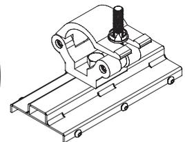
The **FLOORSTANDS FOR FLATMAX** are entirely made from aluminium and are suitable to position FlatMax screens on to the floor.
