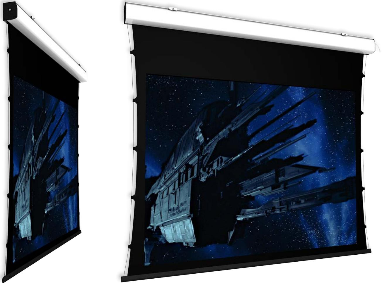
**COMPACT TENSIONED** is a motorized screen that incorporates a tab guide cable system which maintains tension on the cloth in order to get the screen surface perfectly flat. This product has been specifically studied for the niche of the Home Theatre market, so it is the right solution for the most demanding requests. It is professionally masked with black curved side borders and a black top border of 30 cm.
