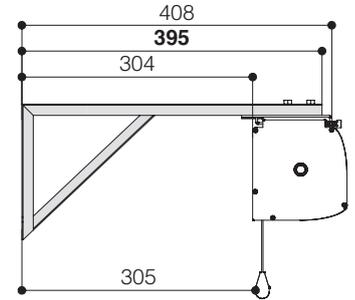
**FALSE CEILING MOUNTING SET** is a set of brackets which is suitable to lower a Compact or Major screen housing up to 100 cm. from the ceiling. It is an ideal accessory to suspend a screen from a high ceiling. The threaded rods can be cut at the desired length.
